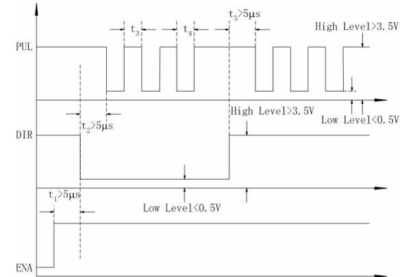
Figure 12: Sequence chart of control signals
