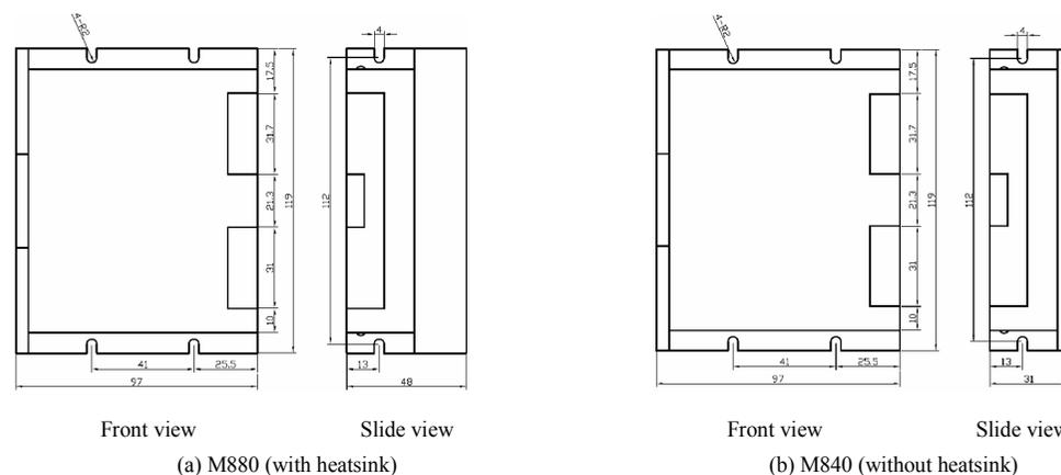
Figure 1: Mechanical specifications
