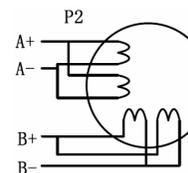
Figure 9: 8-lead motor parallel connections
